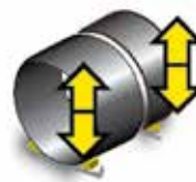
Joining of shell sections using roller beds with hydraulic fit-up system. Internal and external submerged-arc welding performed by a column and boom station.
